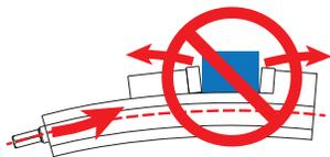
Other vises have screws on the bottom of the vise creating uneven torque in the jaws.
