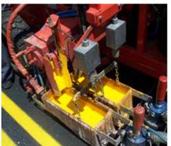
Thermoplastic pavement marking compounds have long been used on the world's highways. The long-term performance, cost benefit and wide range of application techniques provide customers an enduring marking solution while improving motorist safety.
