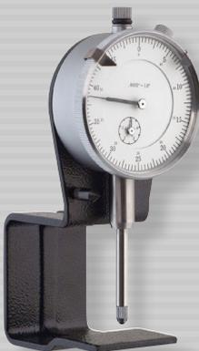
*Dial Gage is designed to check wearing of disc rotors. Also used to determine deviation in thickness of rotors as well depth of disc-scoring caused by worn brakes.*
